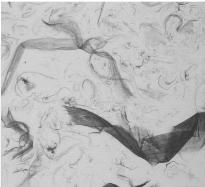
Aqueous MIRALON® Pulp Dispersion showing "Sheetlets"
