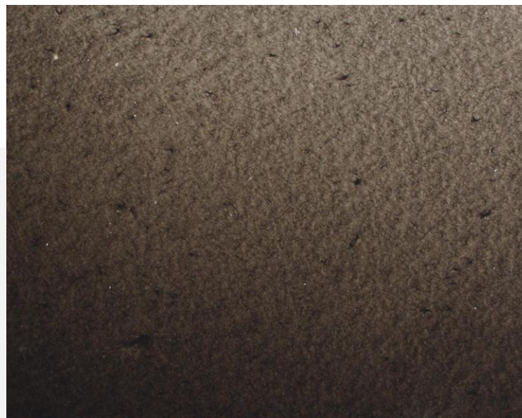
NMP Masterbatch: 1.25% MIRALON® Pulp, 3.75% PVDF.
