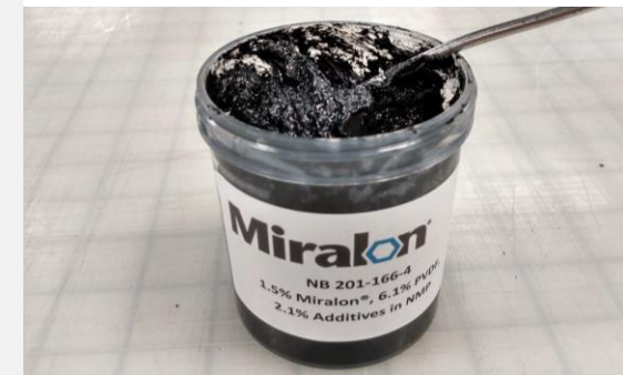
The pulp is combined with a binder and solvent to make a Masterbatch
