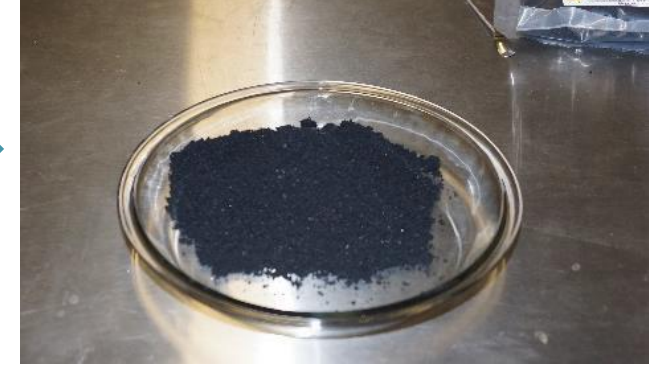
Dispersible Pulp made by standard paper processing methods
